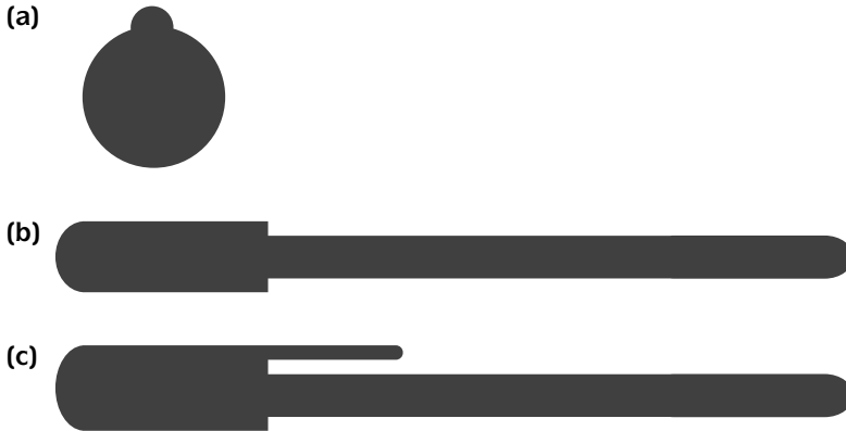
Figure 8.8: Principal component analysis of a pen. (a) Pen looked at end-on. No principal components have been resolved. The pen is not recognisable. (b) Pen looked at sideways with clip obscured. The first principal component is resolved; we can see that the object is “long” and wider at one end, but that the clip is obscured. (c) Pen looked at sideways showing clip; it should be recognisable as a pen. The second principal is resolved; we can now see that the clip and the object is recognisable as a pen. Even in (c), some information is lost. We do not know that the pen is round; it could be a square pen.
